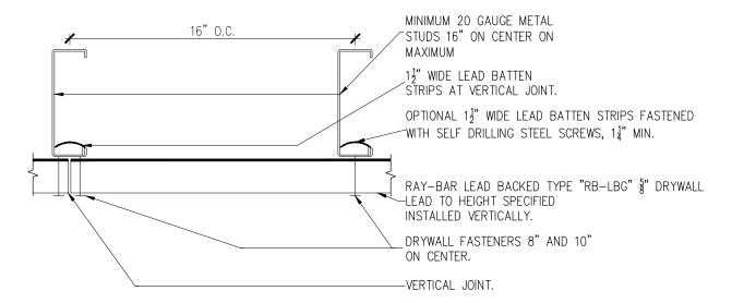
LEAD THICKNESS AS REQUIRED ON RADIATION PHYSICIST SHIELDING REPORT.
